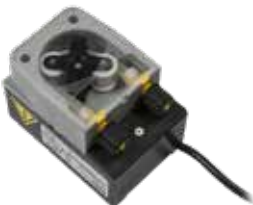
OS0706 Rinse aid peristaltic pump model NBR 0.4 flow rate reg. t/p: 0.4 l/h pressure: 3bar Power supply: 230V- 50Hz complete with: ▶ 2 m suction pipe ▶ 2 m delivery pipe, s/steel bottom weight and filter, injection connection with non- return valve for rinse aid ▶ ROHS certification
