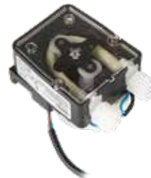
OS1987 Detergent peristaltic pump model NBR 3 flow rate reg. t/p : 3 l/h pressure: 0.1 bar Power supply: 230V - 50 Hz complete with pipes and connections ROHS certification
