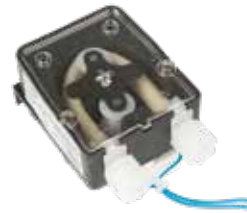
OS1986 Detergent peristaltic pump model PG 3 flow rate: 3 l/h pressure: 0.1 bar Power supply: 230V - 50/60 Hz complete with: 4 m PE tube 4x6, filter and bottom weight, passwall ROHS certification
