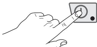
The indicator light of the ON/OFF button "A" (Figure 14) comes on, indicating that the dishwasher is powered and that water is being introduced and heated.
