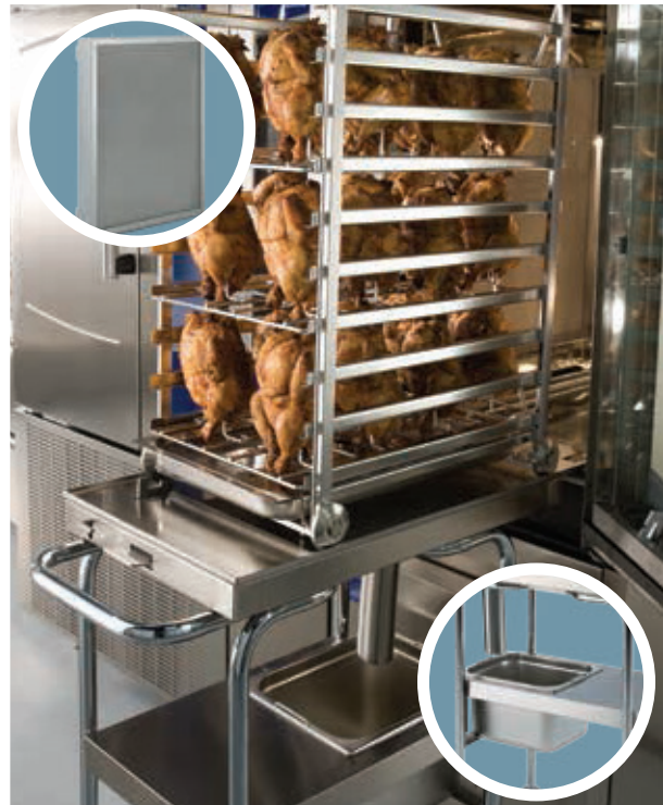
Fat filter and grease collection trolley
