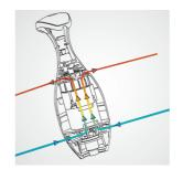
**Air cooling system** permits to work longer without overheating.
