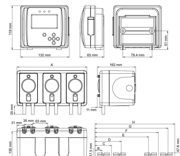
2 pumps 3 pumps 4 pumps 5 pumps 6 pumps Dimensions A B 196 293 391 489 586 42.5 24.4 42.5 24 42.5 C D E F N/A 103.5 85 103.5 103.5 164.5 164.5 164.5 85.3 225 N/A N/A 281 318 336.5 N/A N/A N/A 379 397.5 G N/A N/A N/A N/A 458 Н 110 207 305 403 501 Weight 4 kg 4.5 kg 5 kg 6 kg 7 kg
