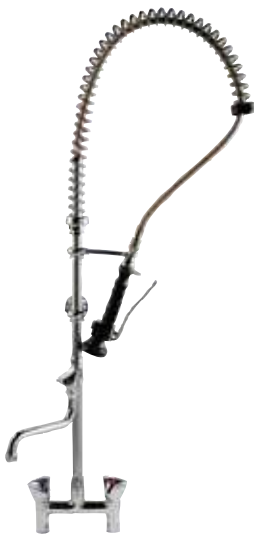
Two hole mixer tap with shower unit with swivel, water supply and base connection Ø3/4", spout of mixer tap L=305mm H=340mm
