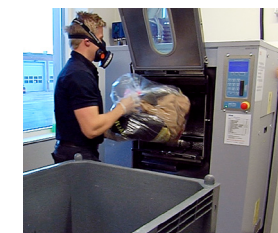
3. Bring the laundry bags into the "Red area" in the laundry and fill the barrier washer. Start the approved program.
