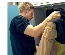
5. The clean and re-impregnated safety equipment is dried in a special designed drying cabinet.
