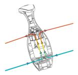
Air cooling system permits to work longer without
