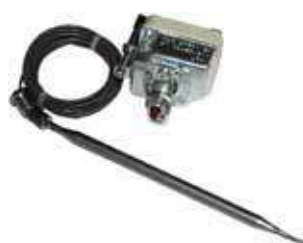
OS1933 Thermostat monophasé 220 °C bulbe Ø6x133 mm capillaire 2020 mm 16A 250V
