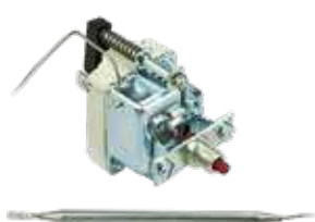
004912 Thermostat monophasé 130 °C bulbe Ø6x130 mm capillaire 870 mm 16A 250V
