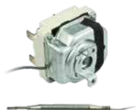
OC1000 Thermostat monophasé 210 °C bulbe Ø6x75 mm capillaire 1250 mm 0.5A 12V
