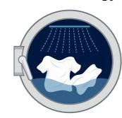
Water is showered from the top of the drum, effectively wetting the laundry with minimal water usage. This unique spin shower wash mechanism enhances washing performance while conserving water.
